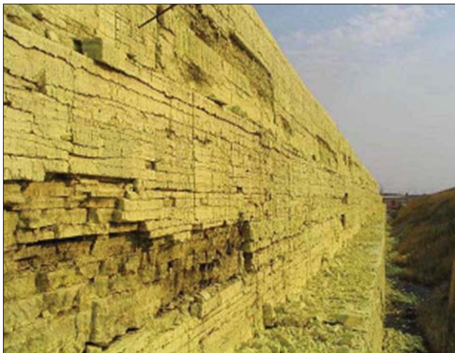
This sulfur block shows weathering after an intermediate storage period (Fig. 2).
